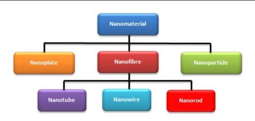
Figure 4.2 Schematic representation of types of nanomaterials based on shape
